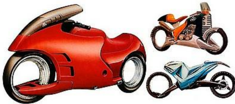
Going Hubless. The hubless wheel was invented by Franco Sbarro, who incorporated it into the Sbarro Osmos car in 1989. He also built at least two motorcycles employing the hubless technology.
